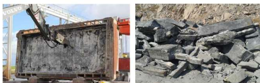
Figure 2. Images of spent pot lining of the Al production process 5 .
